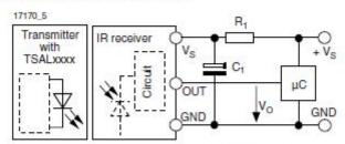
$R_{_1}$  and  $C_{_1}$  are recommended for protection against EOS. Components should be in the range of 33  $\Omega$  <  $R_{_1}$  < 1 k $\Omega,$   $C_{_1}$  > 0.1  $\mu F.$
